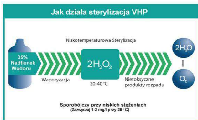
Picture 1. Schem of decontamination using STERIS VHP® system
