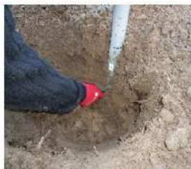
Fig. 1. Measuring procedure in sequence: Sticking PVC pipes in the ground, sampling, pouring oil through the sample, the analysis of soil samples.
