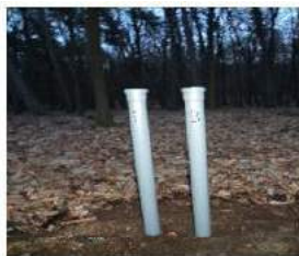
Fig. 1. Measuring procedure in sequence: Sticking PVC pipes in the ground, sampling, pouring oil through the sample, the analysis of soil samples.
